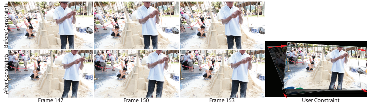
Figure 8: Before region constraints were applied (top row), the frame is skewed. The region constraint is drawn on frame 150 and it corrects for this deformation. The red arrows show the change in the quadrilateral drawn in white for the region constraint. After the video is stabilized with the constraints, note that the neighboring frames are corrected appropriately as the background is upright and there are fewer distortions.
