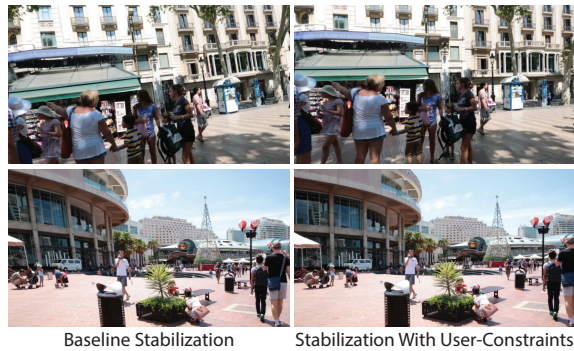
Figure 9: Comparison of initial baseline with result using user constraints. In all examples on the left, the baseline stabilization is not satisfactory as the scene is distorted and the horizon is not level. The same frames in our result are less distorted as the structures are vertical.
